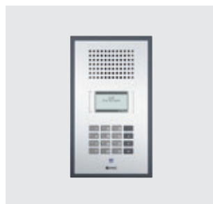
WS 800P | LCD display, Full keypad
